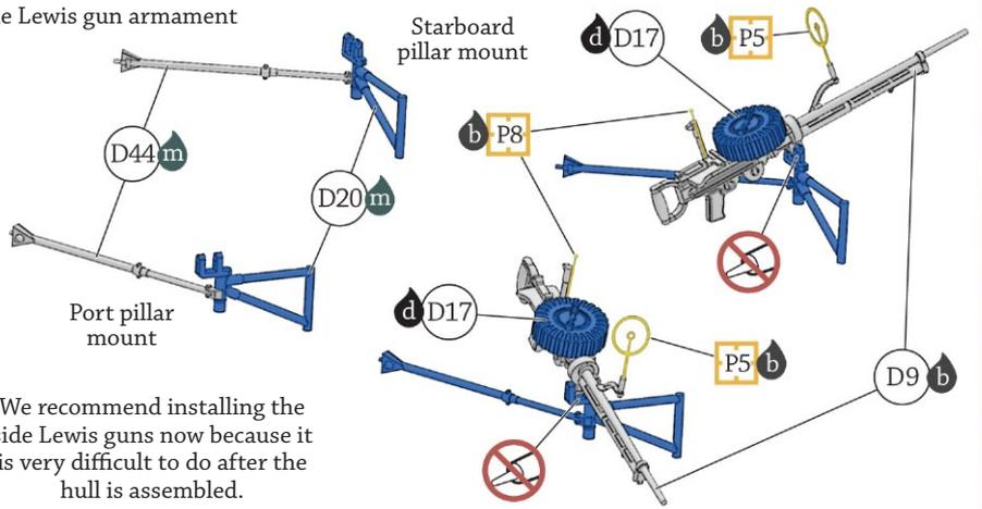
We recommend installing the side Lewis guns now because it is very difficult to do after the hull is assembled.
