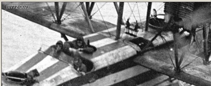
Cockpit coaming detail from converted early production Felixstowe F.2a N4297 **B2**. Note the petrol pumps, square hatch for the engineer, Scarff ring on the rear coaming and smaller Scarff ring on the bow.
