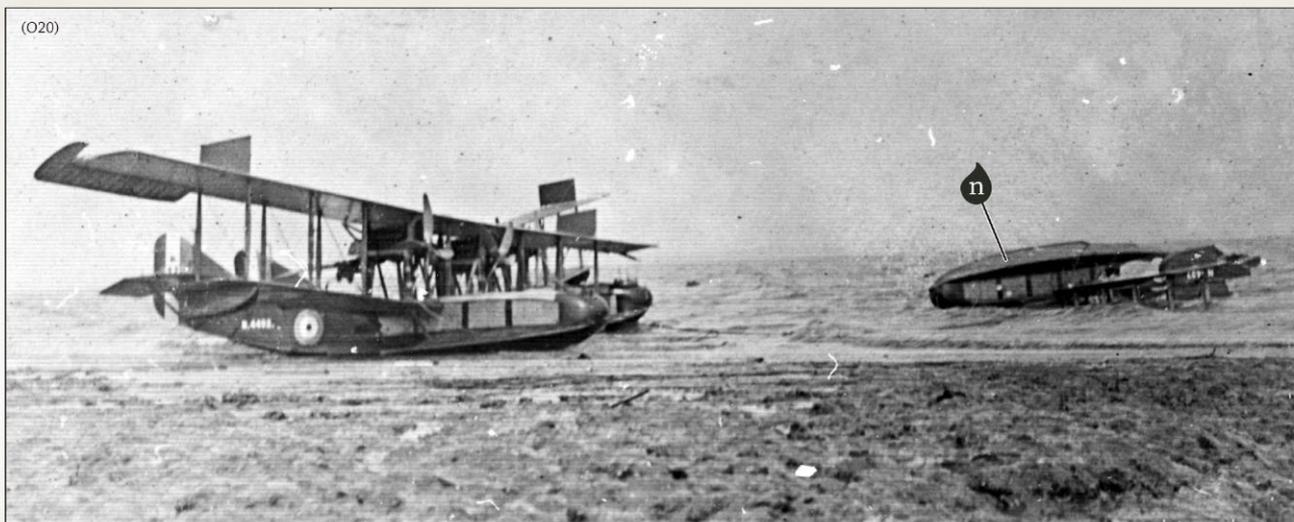
Three unidentified late production Felixstowe F.2a, one of which is looking decidedly the worse for wear, that all appear to be from a production order placed with May, Harden & May (numbers N4480 to N4504). Note the open cockpit and balanced ailerons on the closest boat and dark hull bottoms.
