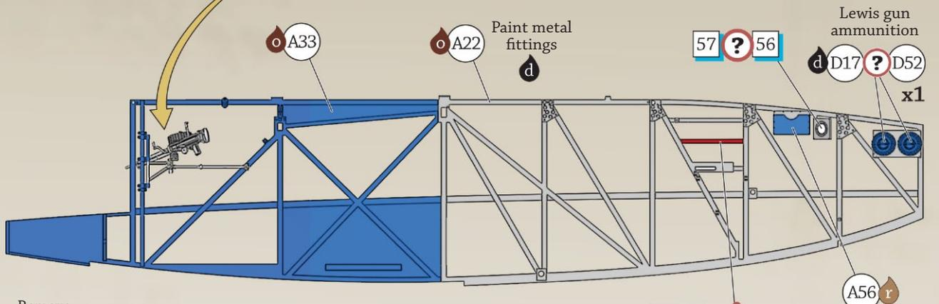
Remove switches if installing **A1** between pilots seats
