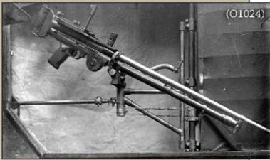
Starboard hull Lewis gun and mount from an unidentified F.3 (not F.2a). Note that the ring **P5** and bead **P8** sights are not fitted. The pillar mounts allowed the guns to be stowed internally until they were required.
