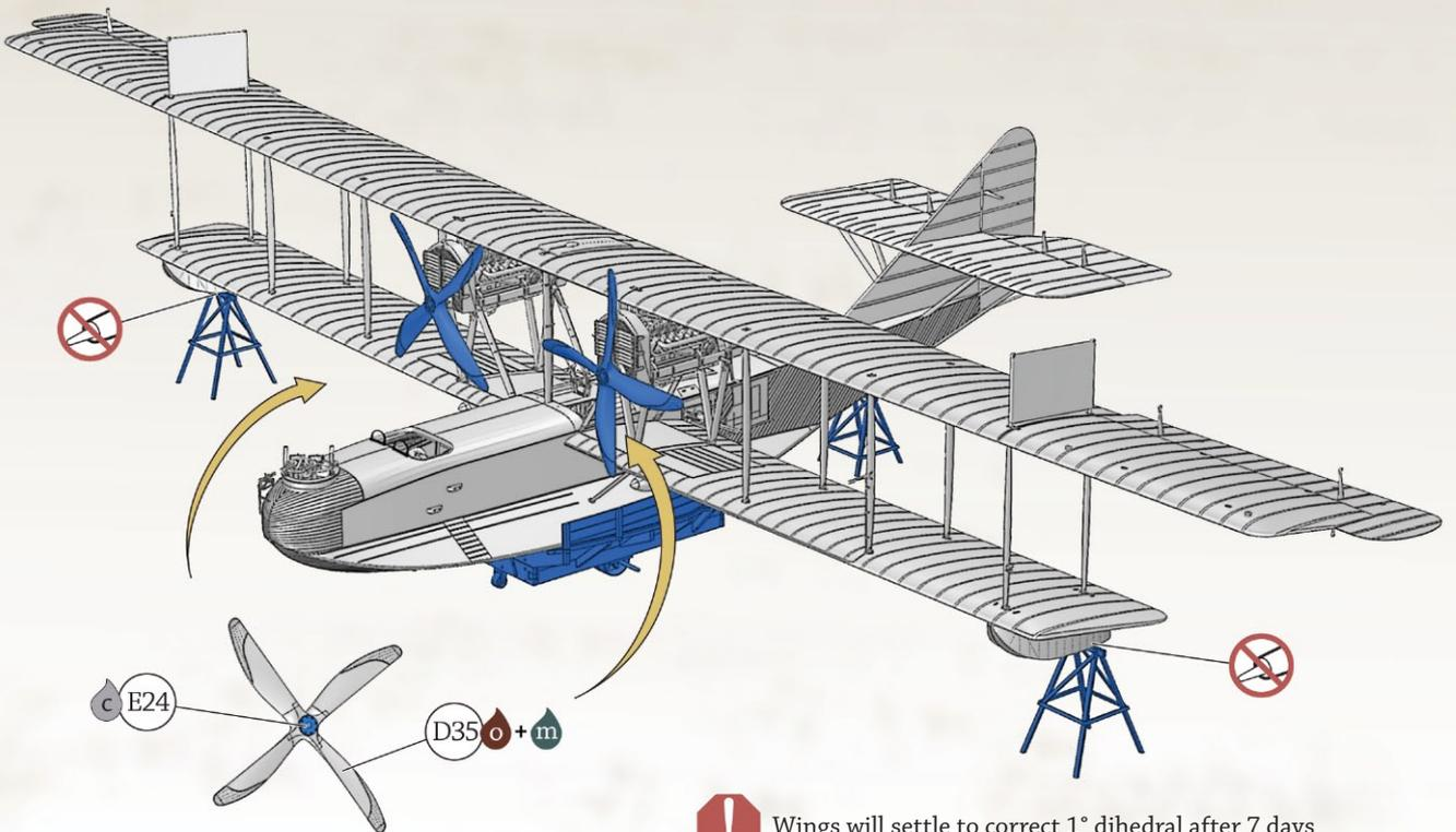
Counter-clockwise rotating propellers
